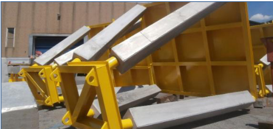
Fig. 1 - Anode pods with aluminium alloy – 300 kg anodes
