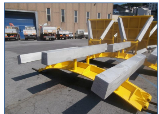
Segment of clamp with galvanic anodes (monopiles, single point moorings, etc)
