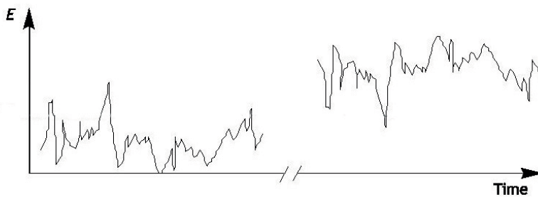
Fig. 2 - Interference scheme from non-stationary continuous stray currents in case of a metallic structure embedded in concrete
